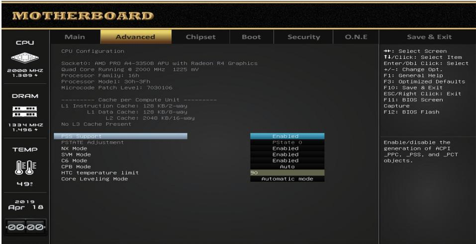
The screenshot shows the BIOS Motherboard Advanced menu. The CPU section is expanded, displaying the following information:
